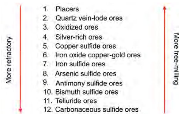
Figure 2.1 Gold ore types based on mineralogical characteristics
