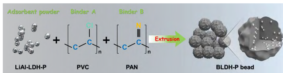
Figure 4.1 Schematic illustration of the fabrication strategy for BLDH-P beads.
