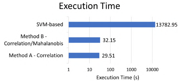
Figure 4.21: Execution time for method A and B, and SVM-based approach (representation in logarithmic scale).
