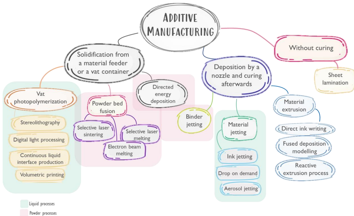
Figure 2.2. Additive manufacturing technologies classified according to the type of process.
