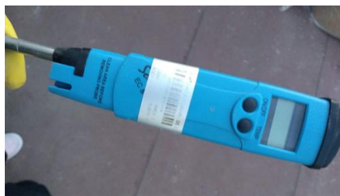
Figure 9. Equipment used for conductivity measurement
