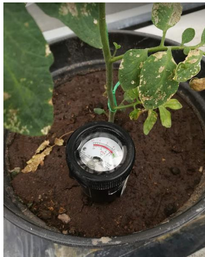
Figure 7. Equipment used for pH measurement in a tomato pot.
