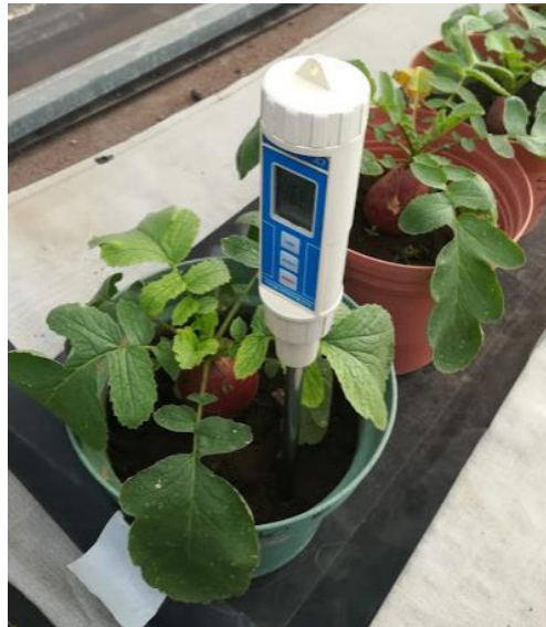
Figure 8. Equipment used for humidity measurement in a radish pot
