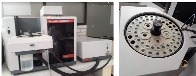
Figure 14. Atomic Absorption equipment used for the AsT measurement
