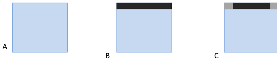
Fig. 4 - A: glass coverslip; B: glass slip with the resistive ink printed on it; C: conductive contacts placed over the resistive ink.
