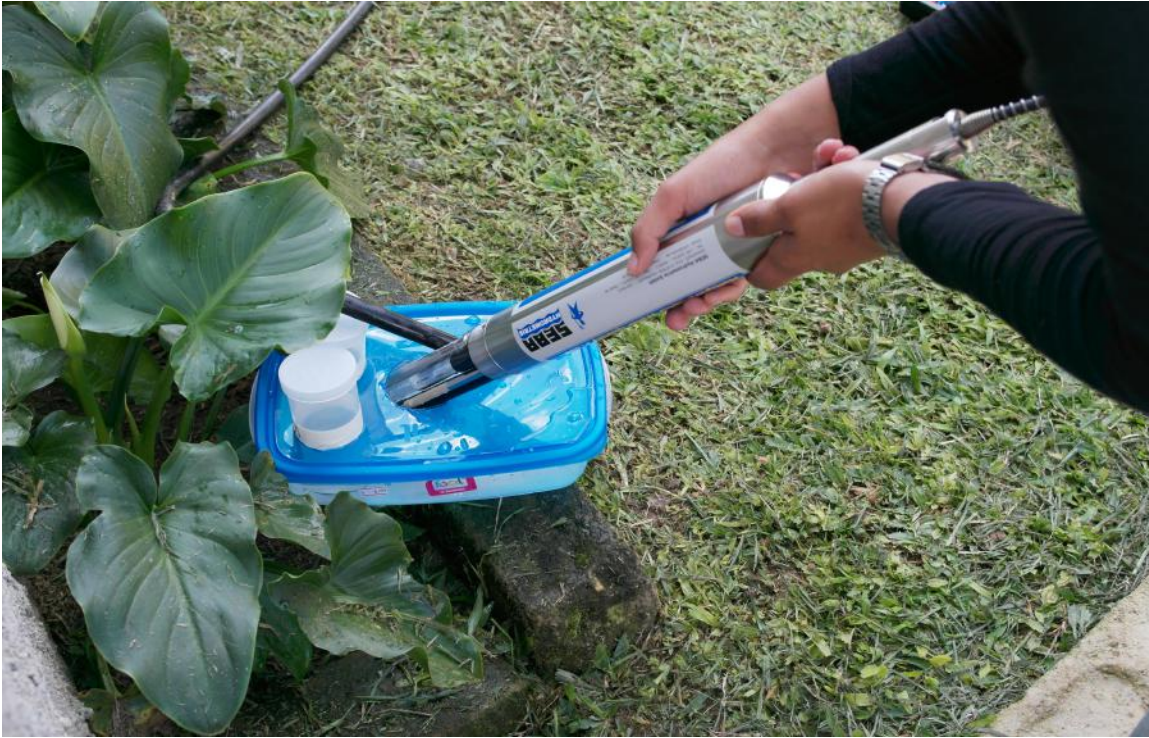
Figure 19.: Flow-through chamber for groundwater sampling
