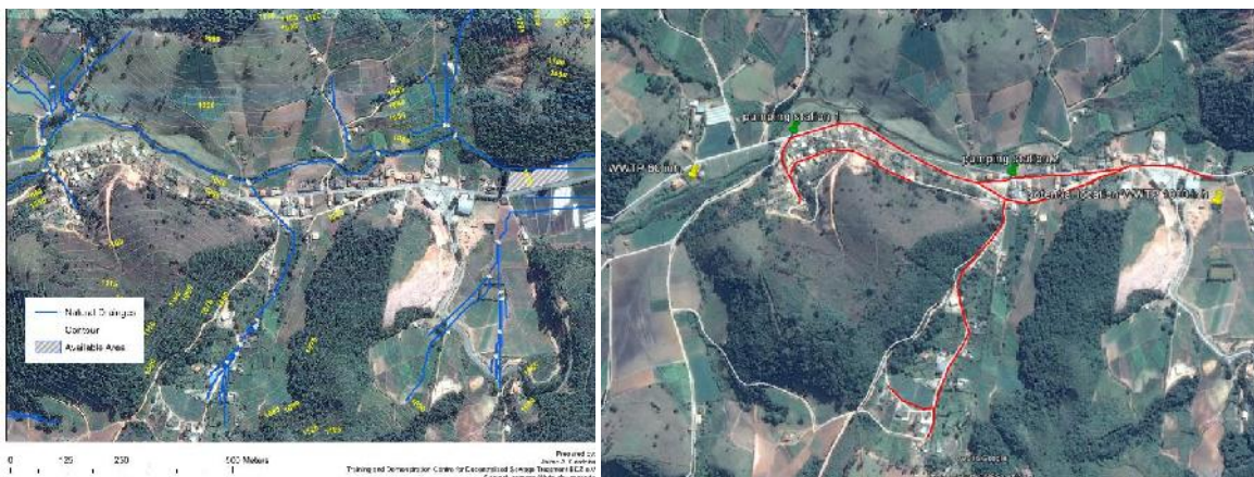
Map 5: Map of Barracão dos Mendes showing the natural drainage areas (left) and the projected sewer network base on gravity flow (right). Source: BDZ e.V.
