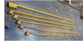
Figure 12: Phases of bows in construction and made from pau-brasil
